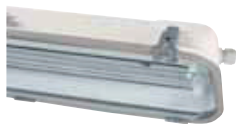
Painted steel-polycarbonate lighting fixtures with symmetrical reflector in aluminium, for T8 tubes 230V IP66
