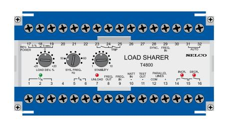
The T4800 calculates I x cos  $\phi$ , representing the active load. The load on each generator is compared with the load on the other generators. Contact signals for increase and decrease with proportional pulses are obtained as output. These pulses regulate the frequency and load via the electric servomotor on a conventional speed governor, or by controlling an electronic speed controller via an intermediate E7800 Motorized Potentiometer.
